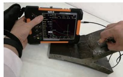
● Angle weld testing
